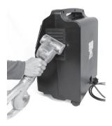
**Detail steps:** Loosen the screw and remove the filter grid.
